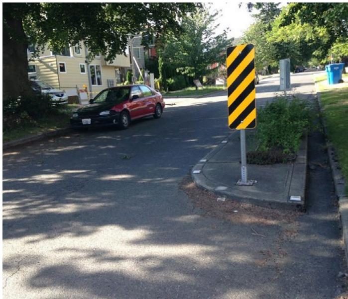
Narrowing of roadway with lateral extension of the curb into the street or islands on both sides of the street at a midblock location. Edge islands can leave area along the curb line open for bike lanes and/or existing drainage. In some cases, travel width may be reduced to force motorists to a single lane to take turns to pass through pinch point. This treatment may be combined with a mid-block crosswalk to reduce crossing distances and improve pedestrian visibility.
