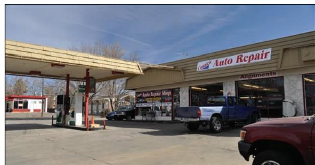
This large gas station with three service bays and a matching canopy over the pump islands, was originally designed in a Rustic Modern Style with residential materials including cedar shake shingles on the shallow mansard style fascia with field stone-clad walls. The sensitive relationship of the wood to the stone is obscured by paint. The stone could be stripped and the shingles would need to be replaced.
