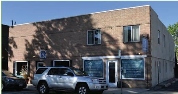
This contractor-designed building, likely the joining of two older buildings unified by a brick facade, reflects a mediocre standard of design and workmanship. The east half of the building is two stories while the west half is only a single story, hidden behind a two-story false front.
