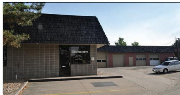
This modest garage is marginally Modernist, having stucco walls and a flat roof alongside a later functional addition built in gray concrete bricks. The two distinct parts are unified by a shingled mansard-style fascia. The building retains its automotive use.
