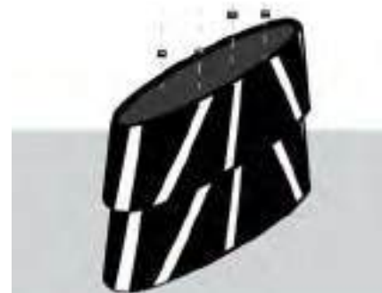
Figure 7 - Place on top the second planter. Tighten the last nuts with the socket wrench.
